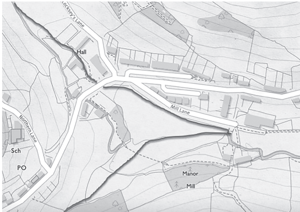
Figure 4. Probable courses of the northern and western valley streams before they were made into leats.
